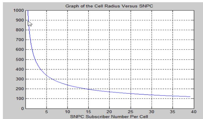
Figure (3) – Cell Radius (meter) Vs. SNPC
